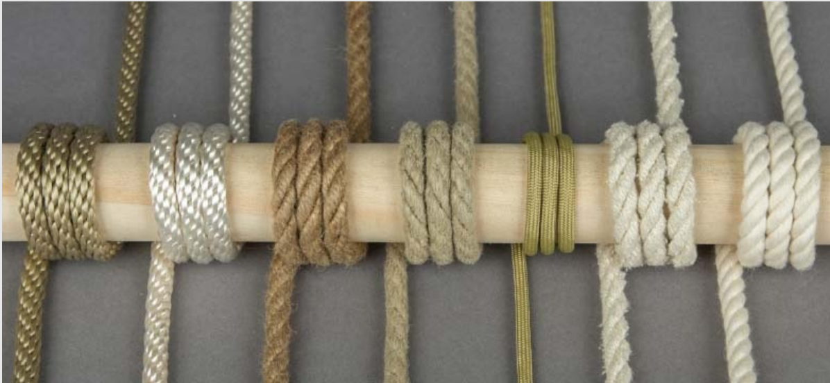
(From left to right) Multifilament Polypropylene (MFP), Nylon, Jute, Hemp, Paracord, Silk, Cotton
